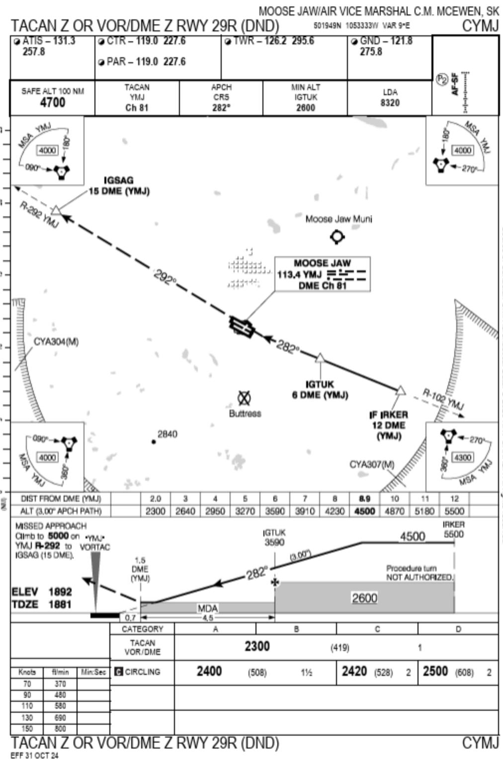
The simplest of TACAN approaches, this one would be flown by being given radar vectors by Terminal to intercept the 282 radial to the Moose Jaw TACAN. Unlike an ILS you don't have glideslope information so there are two ways you could fly this approach vertically: "dive and drive" or Constant Descent Angle (CDA).
